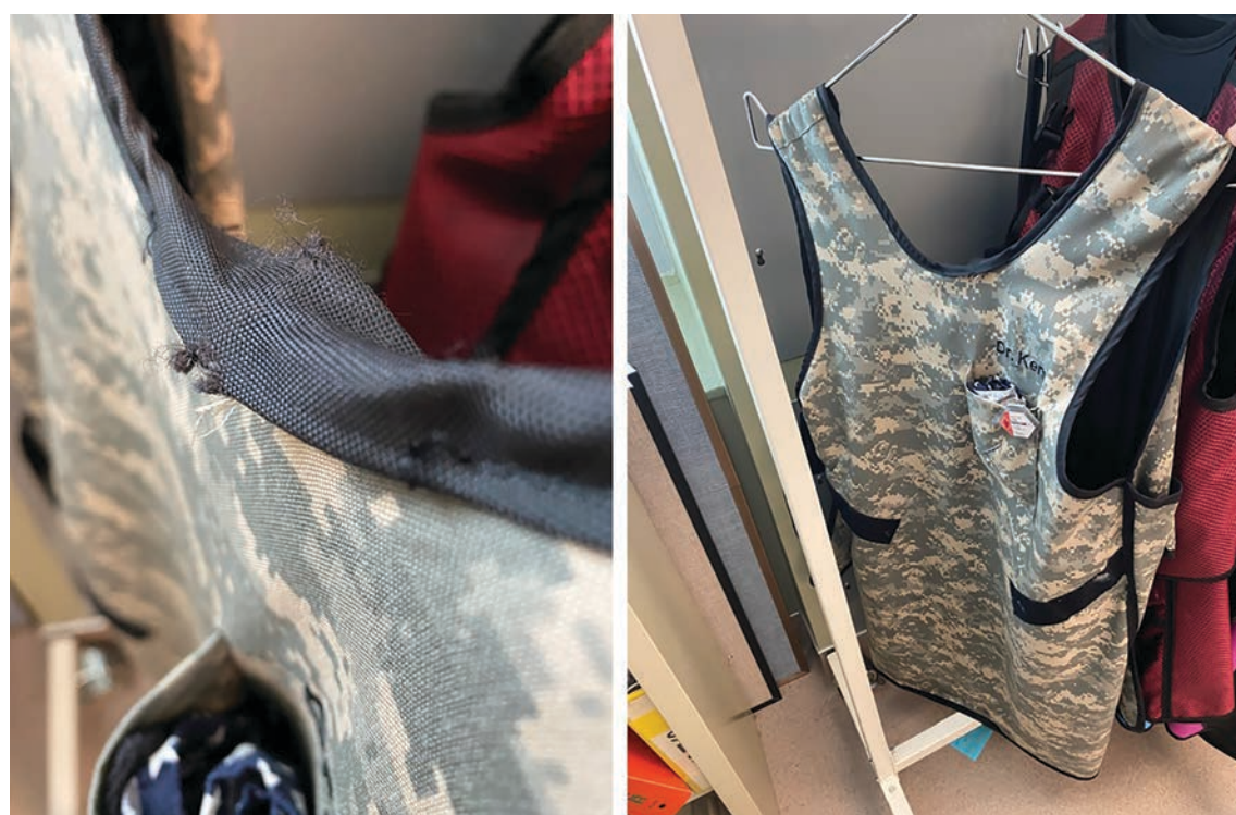
Figure 1. Lead apron showing tears in fabric at neck from frequent use, despite correct hanging on the lab's lead rack.
