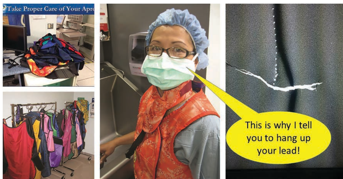
Figure 2. Top left, lead aprons piled up. Bottom left, correct method of hanging lead aprons. Far right panel shows an x-ray image of cracked lead. Our tech reminds us of why we hang lead.
