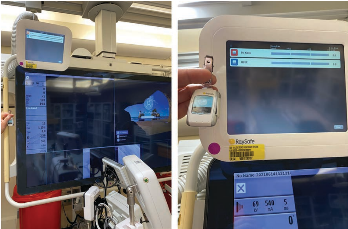
Figure 5. RaySafe radiation real-time radiation monitor (Fluke Biomedical). Each member of the team wears a badge that transmits the dosage to the display for all to see and take appropriate steps to reduce exposure.
